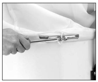
**Figure 14.** Securing the upper bag threaded band clamp.
